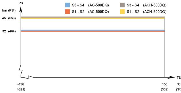
**AC500DQ / ACH500DQ - UL approval pressure/temperature graph\***
