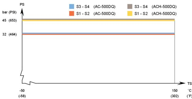
**AC500DQ / ACH500DQ - CRN approval pressure/temperature graph\***
