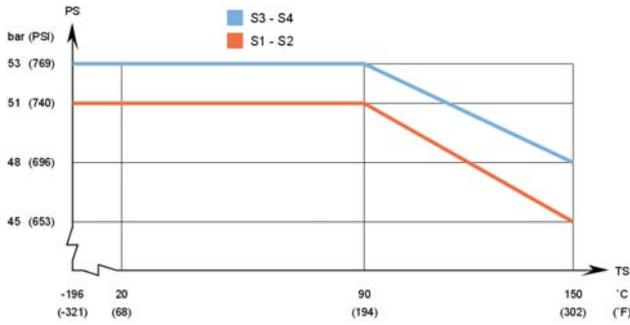
**AC232DQ / ACH232DQ - KHK approval pressure/temperature graph\***
