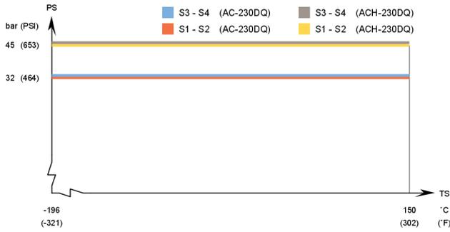
**AC230DQ / ACH230DQ - UL approval pressure/temperature graph\***
