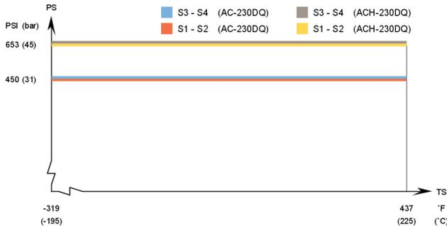
**AC230DQ / ACH230DQ - CRN approval pressure/temperature graph\***
